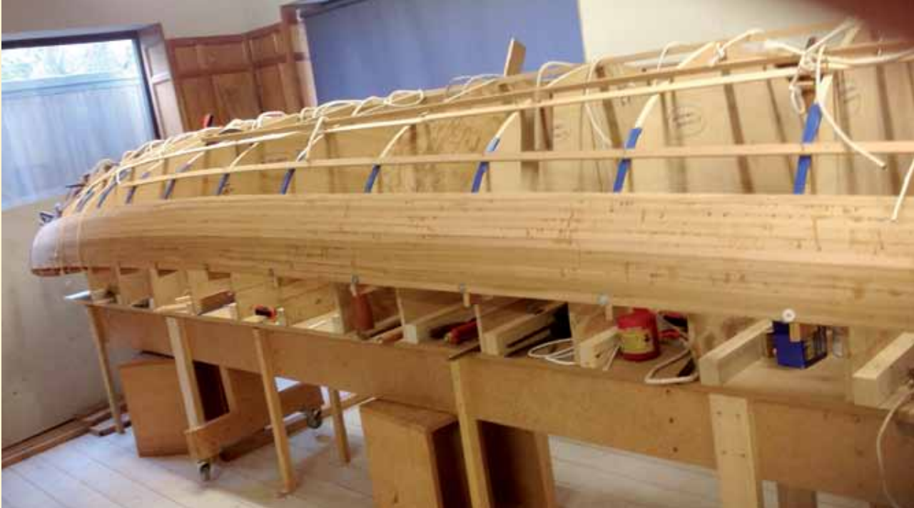
Modern wood construction: building a lightweight rowing skiff using cedar strip planks edge-glued together, often using epoxy... but not always. Photographs: www.cedar-strip.co.uk
