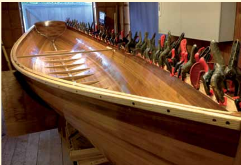
Modern wood construction: building a lightweight rowing skiff using cedar strip planks edge-glued together, often using epoxy... but not always. Photographs: www.cedar-strip.co.uk
