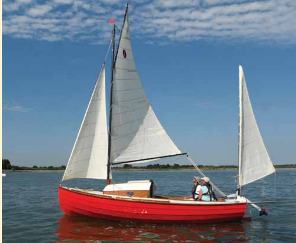
Black carbon-fibre spars reduce weight aloft on this Francois Vivier-designed Jewell, a 22' (6m) trailable clinker plywood gaff yawl.
