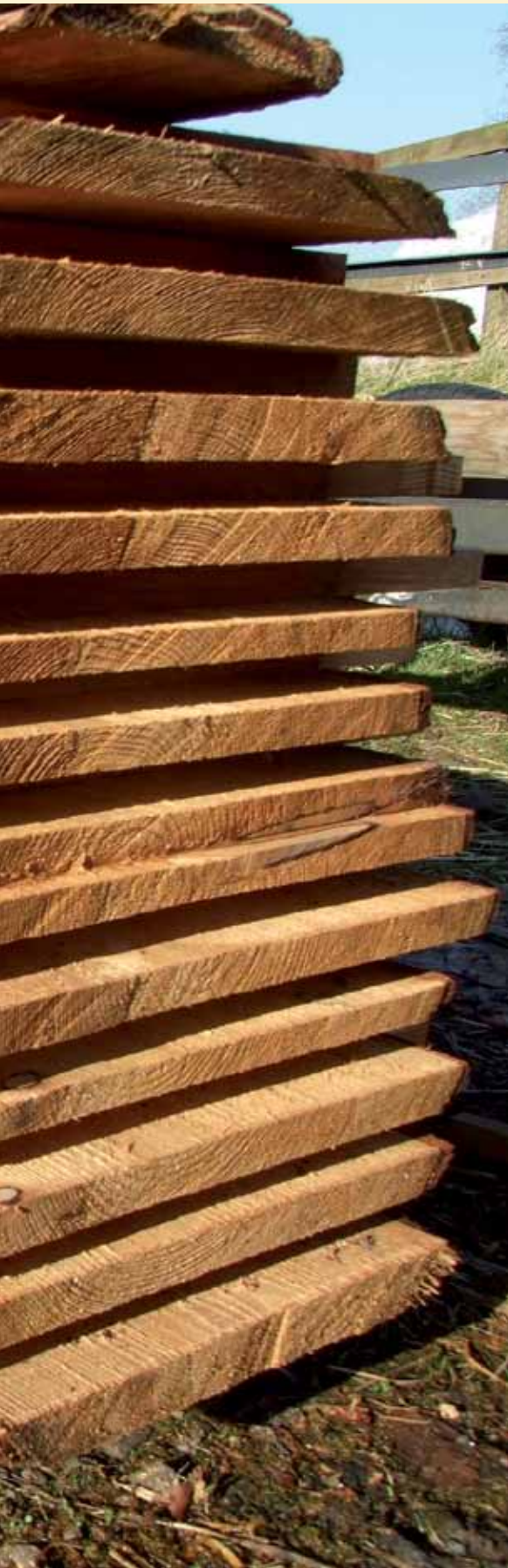
Left: Seasoning Scottish larch 'in stick' at Black Dog Timber. Air drying softwood the traditional way typically takes one year for every 1" (25mm) of board thickness.
